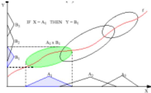
Figure 1 - Mapping Of Input Space Into Output Space<sup>11</sup>
